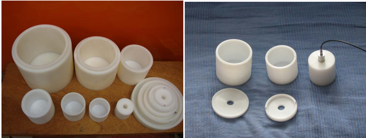
Figure 2: Pictures of the cylindrical shells (left) and the He-3 counter inserted into the 0.2 kg cylinder (right).
